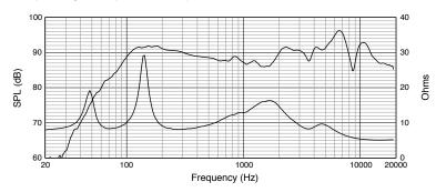
Frequency response in half-space (2pi, mounted in ceiling, 1W, 1m), impedance at  $8\Omega$  (low-impedance) setting; input impedance (lower solid line)
